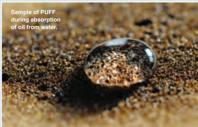
**Sample of PUFF during absorption of oil from water.**
